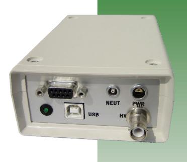
The NScan device is a computer controlled module which measures counts from a counting detector as a neutron detector, a Geiger-Mueller-counter or similar and controls a motor which moves the detector.
