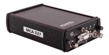
The MCA527 is a battery powered high performance 16K Multi-Channel Analyzer/Multi-Channel Scaler module for gamma spectroscopy (see original data sheet of MCA527). But with upgraded firmware and neutron counting software the same hardware can be used as multiplicity or coincidence counter for neutron counting which picks time intervals between pulses instead of performing pulse height analysis for spectrometry.
