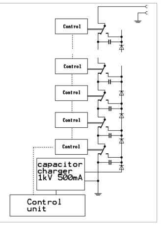
approx. 400ns. The output currents are electronically limited, overcurrent shutdown is staggered over the time.
