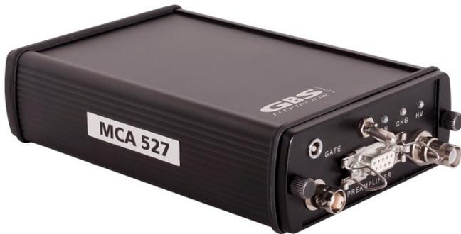
The MCA527 is a battery powered high performance 16K Multi-Channel Analyzer/Multi-Channel Scaler module for gamma spectroscopy (see original data sheet of MCA527). But with upgraded firmware and neutron counting software the same hardware can be used as multiplicity or coincidence counter for neutron counting which picks time intervals between pulses instead of performing pulse height analysis for spectrometry.
