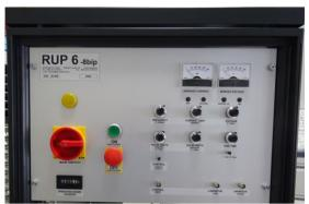
RUP6 is a universal high voltage pulse generator concept, which can be built for voltages from 2kV to 30kV. Prominent features are high pulse current, very high efficiency, scalability of the voltage and ultrafast switch off in case of arcs.
