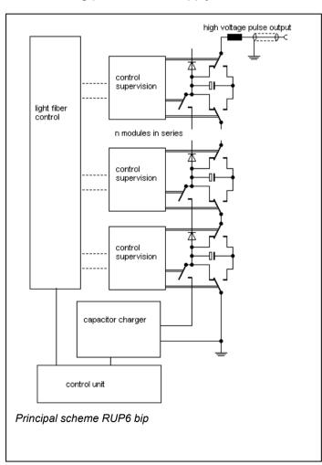
The pulse modules of the RUP6bip contain full bridges instead of half bridges as the standard RUP6 design.
