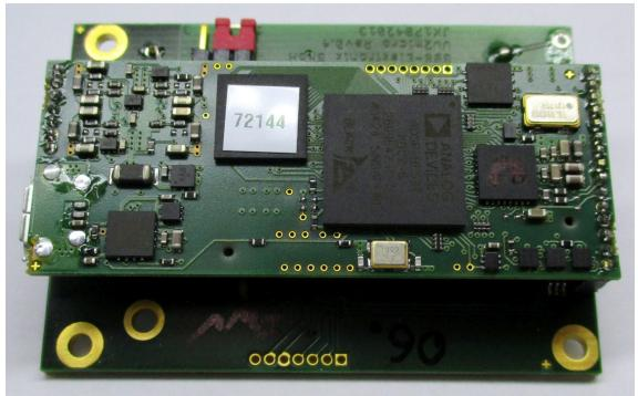
Figure 11: MCA527micro mounted on the amplifier board
