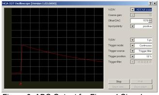
Figure 6: ADC Output for Figure 4 Signals
