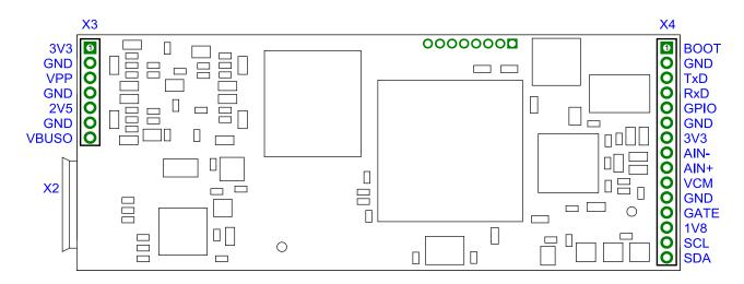
Figure 1: Connection Diagram (Top View)
