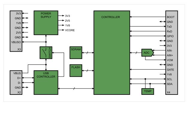
Figure 1: MCA527micro / micro+ Block Diagram
