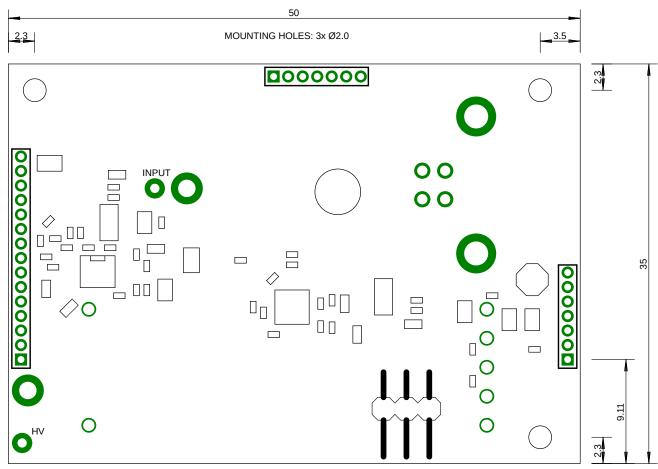
Figure 12: Outline Dimensions of Amplifier Board A-GBS-MCA527MICRO-PA2
