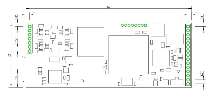
Figure 8: Outline Dimensions (Top View, all Dimensions are in Millimeters)
