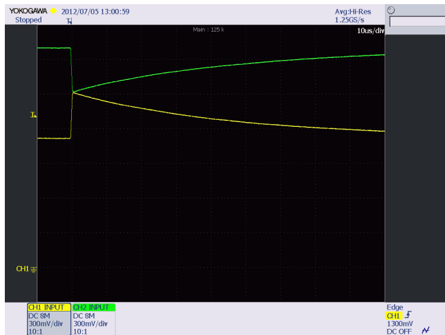
Figure 5: Signals of Differential Driver
